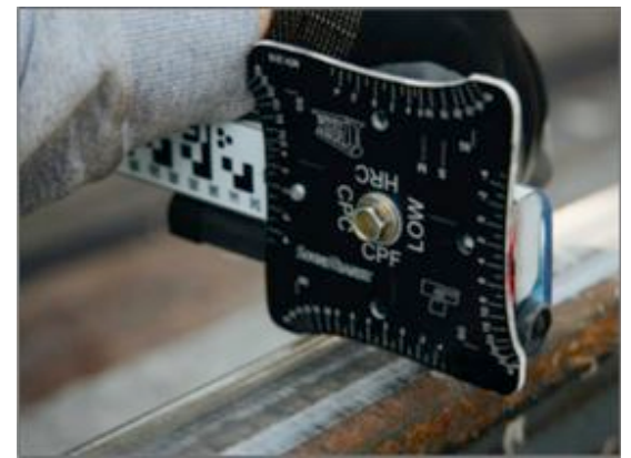
Above, a track inspector checks rail-head profile with a gauge that has different faces for different positions along curves. Rail vehicles experience the best ride and cause the least wear to wheel treads and rails when both have an ideal shape. (Image by Advanced Rail Management)
