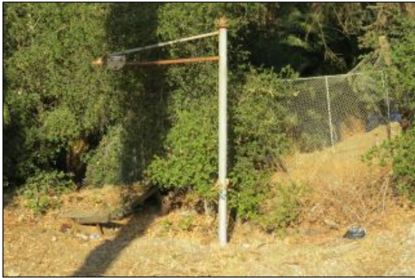
The jib crane near the old water tank can still be turned using the handle hinged on its lower right side, but don't cross the racks to do so.
