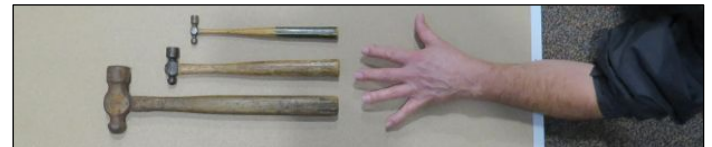
Small ball peen hammers from your editor’s toolbox, and a big one from the Museum’s collection. For industrial applications, powered peening tools are often used.
