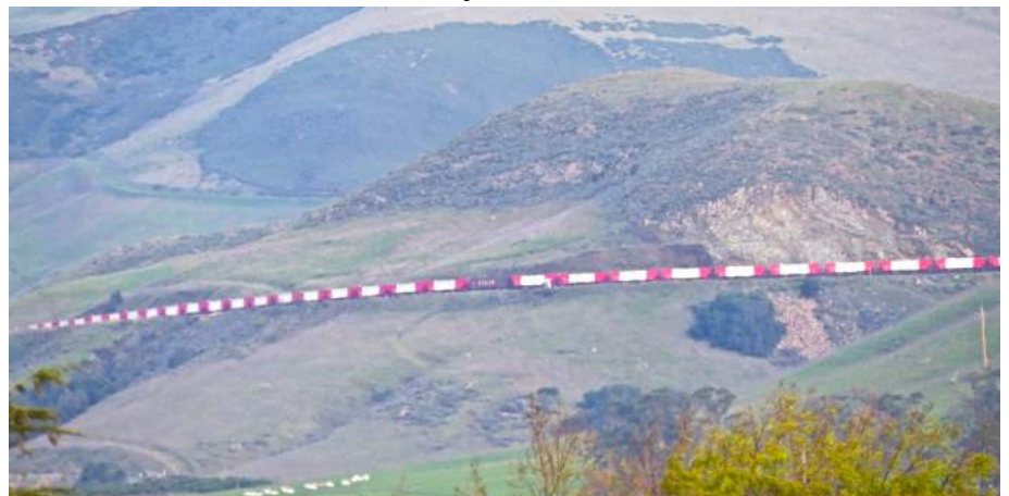
In January U.P.R.R. operated ballast trains along the Coast Route. Here, a colorful set of maintenance contractor Herzog’s hopper cars head north at Chorro siding. Another train of hopper cars with a conveyor belt all along the bottom and special distributors at each end was parked awhile at San Luis Obispo. Photo by Glen Matteson
