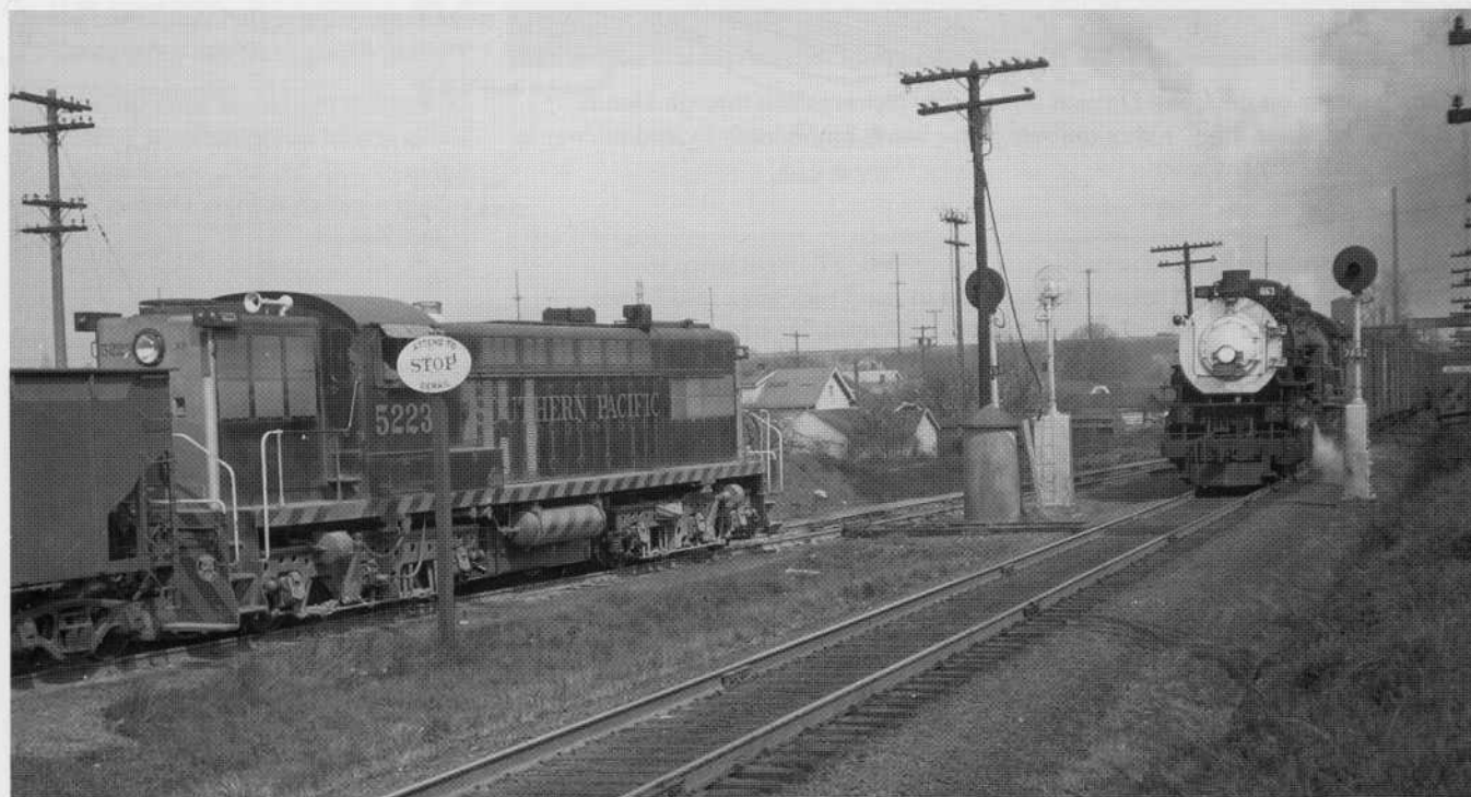
Baldwin 5233, coming off the West Side Branch, stays in the clear for train No. 663 with engine 5031 at Willsburg Jct., Oregon, in 1953. At strategic locations such as this, the concrete phone booths played a vital role in train operations before the advent of two-way radio. -Tom Dill collection
